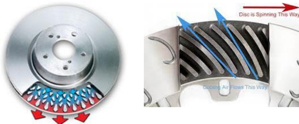
Figure 1: Pillar & Curved Vane Designs Being Studied
